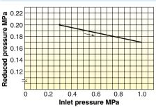
This chart shows variation in reduced pressure when the inlet pressure of 0.3 MPa is changed between 0.3 MPa and 1.0 MPa while the reduced pressure is set at  $0.2\,\mathrm{MPa}$  MPa.
